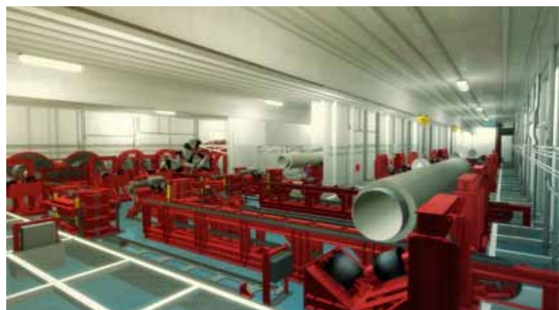
Firing line below main deck
