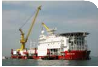
Jascon 30 is a shallow water pipelay construction accommodation vessel with modular S-lay pipelay equipment enabling the barge to combine various offshore construction duties in the oilfield.
