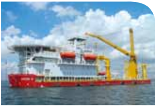
Jascon 31 is a deepwater construction accommodation vessel for both shallow and deepwater operations.
