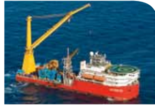
Jascon 25 was built according to the Sea Trucks Group hybrid design philosophy and is one of the Group's four major deepwater pipelay construction vessels.
